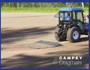
The CAMPEY™ Dragmats come in a variety of different sizes and are available in heavy-duty reinforced rubber or steel construction. Dragmats are ideal for rubbing-in top dressings, dew and clippings dispersal. Small mats can be hand-pulled, while the wider units are more suited to towing on the optional 3-point frame. Available in 4 different widths, and 2 different thicknesses (rubber) for a variety of different handling applications and tasks.
